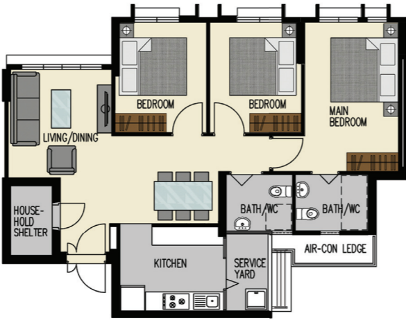
LAYOUT IDEAS FOR 4-ROOM APPROX. FLOOR AREA 94 sqm ( Inclusive of Internal Floor Area of 90 sqm and Air-Con Ledge )
