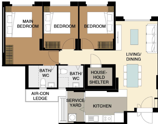
4-ROOM FLOOR PLAN (With Suggested Furniture Layout) APPROX. FLOOR AREA 93 sqm (Inclusive of Internal Floor Area of 90 sqm and Air-con Ledge)
