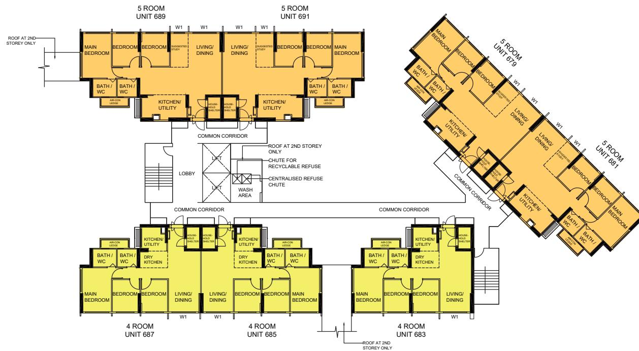
BLOCK 213B | 2ND TO 15TH STOREY FLOOR PLAN
