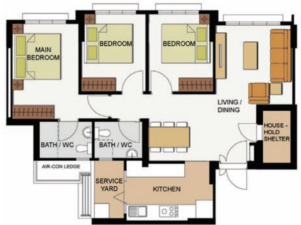
With Kitchen Partition Wall
