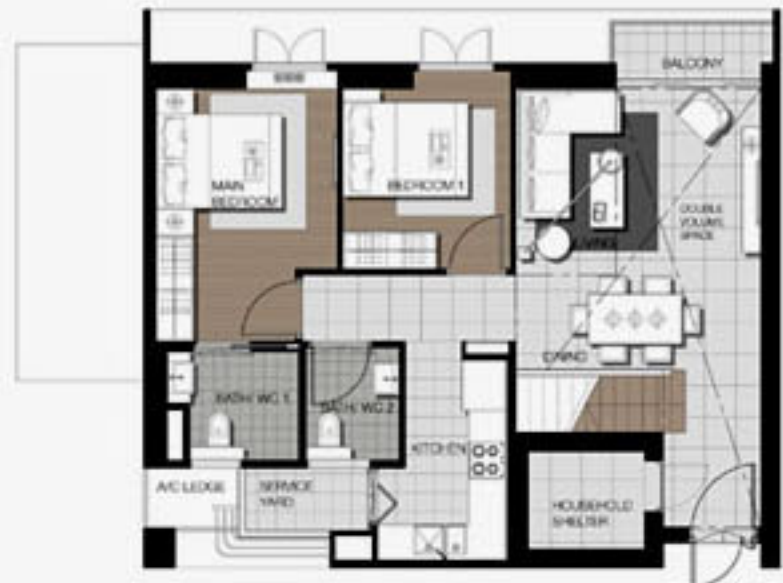
4-ROOM (LOFT 1) LOWER FLOOR PLAN APPROX. FLOOR AREA 109 sqm (Inclusive of Internal Floor Area 88 sqm, Air-Con Ledge and Double Volume Space)
