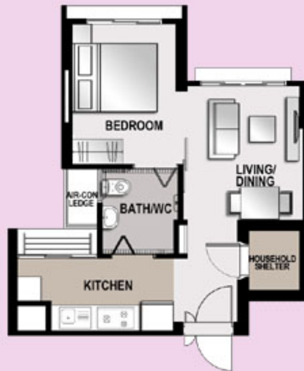
LAYOUT IDEAS FOR STUDIO APARTMENT (TYPE A) APPROX. FLOOR AREA 37 sqm (Inclusive of Internal Floor Area 35 sqm and Air-Con Ledge)
