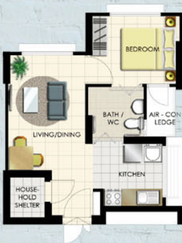
TYPICAL STUDIO APARTMENT (TYPE A) FLOOR PLAN APPROX. FLOOR AREA 37 sqm (Inclusive of Internal Floor Area 35 sqm and Air-Con Ledge)
