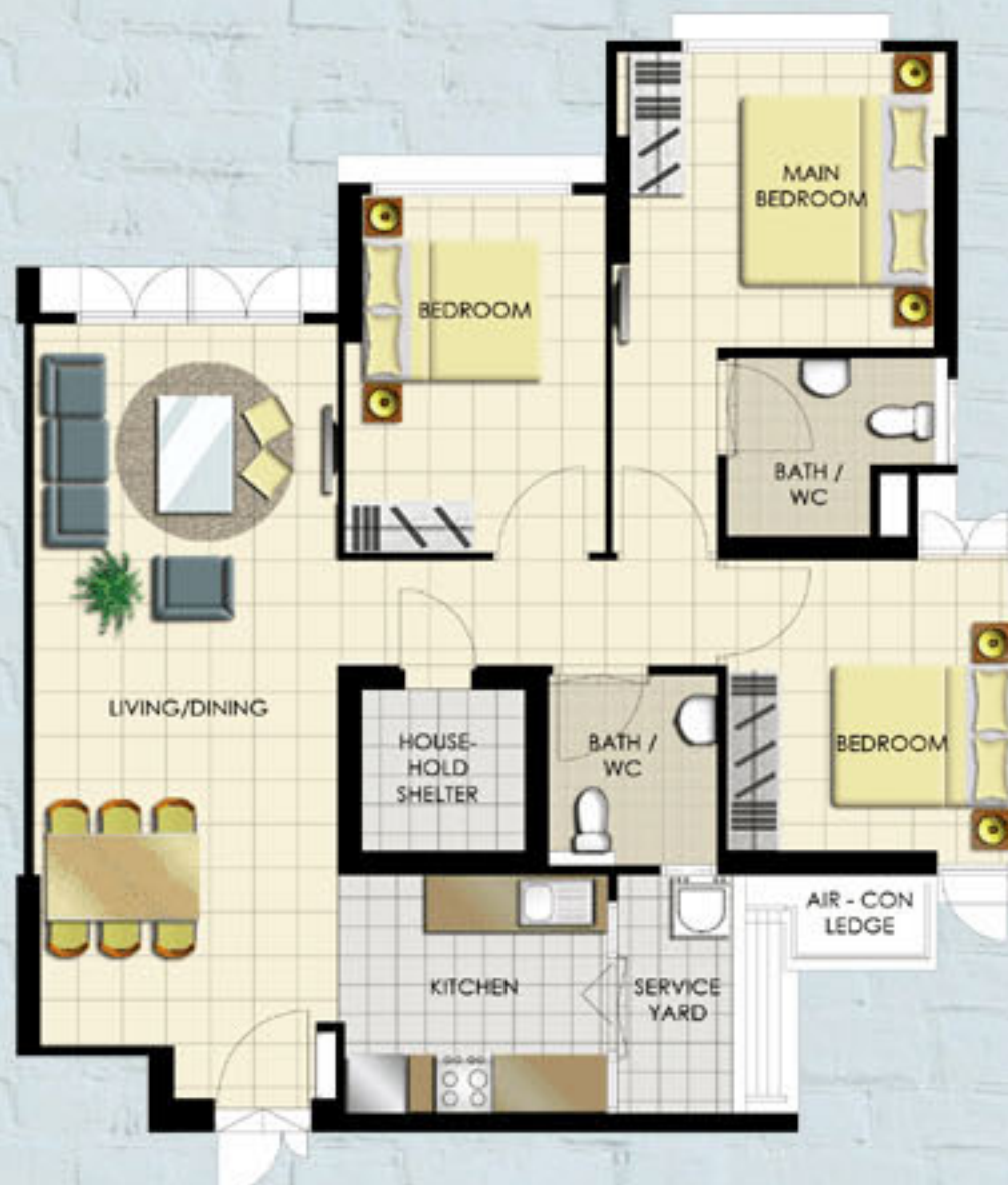
TYPICAL 4-ROOM FLOOR PLAN APPROX. FLOOR AREA 92 sqm (Inclusive of Internal Floor Area 90 sqm and Air-Con Ledge)
