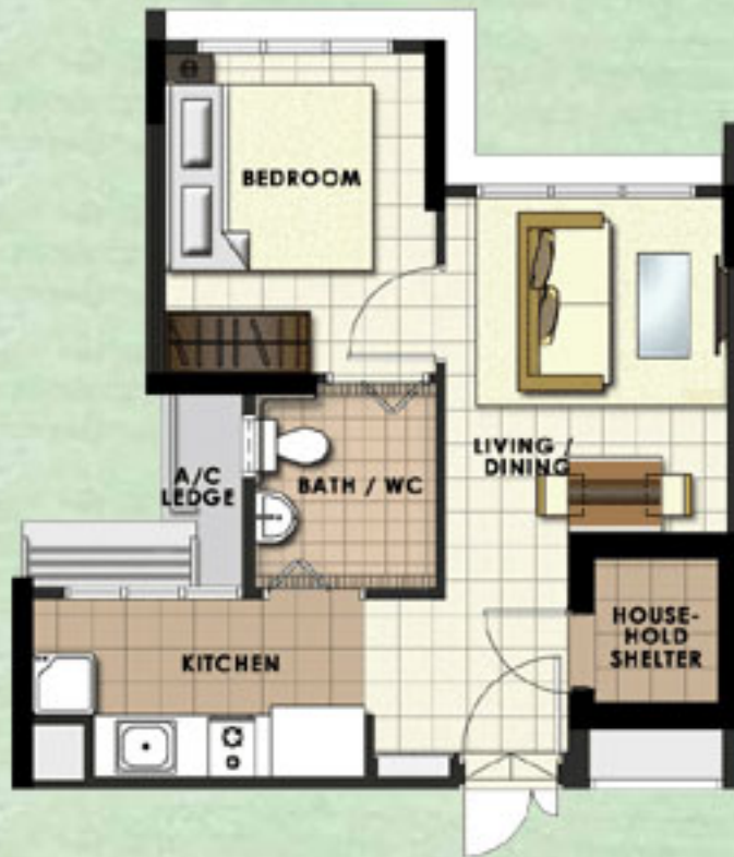
TYPICAL STUDIO APARTMENT (TYPE A) FLOOR PLAN APPROX. FLOOR AREA 36 sqm (Inclusive of Internal Floor Area 35 sqm and Air-Con Ledge)
